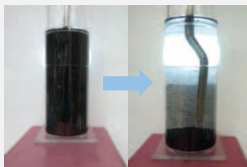
Fig. 3: Dispersion of powder to be flocculated by an add-on of poly-electrolytes
