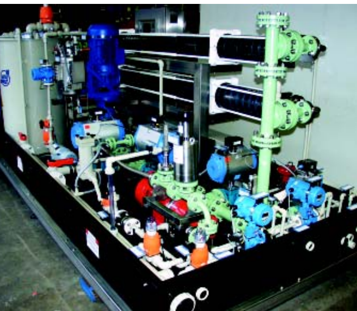
Quite versatile – mobile membrane plants recover the acids flexibly exactly where they accrue
