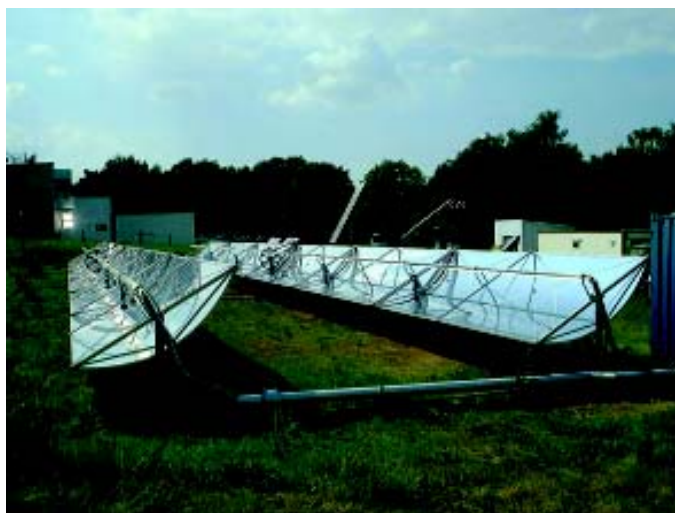
Steam jet cold and parabolic through collectors for innovative cold production (Source: DLR Köln-Wahn)
