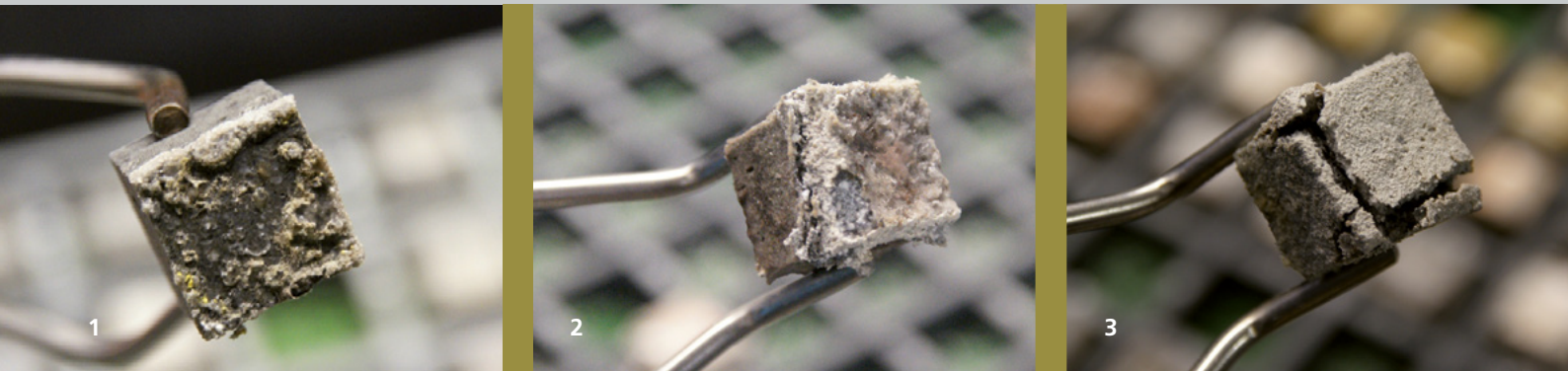
1–3 Weathered test cubes.
