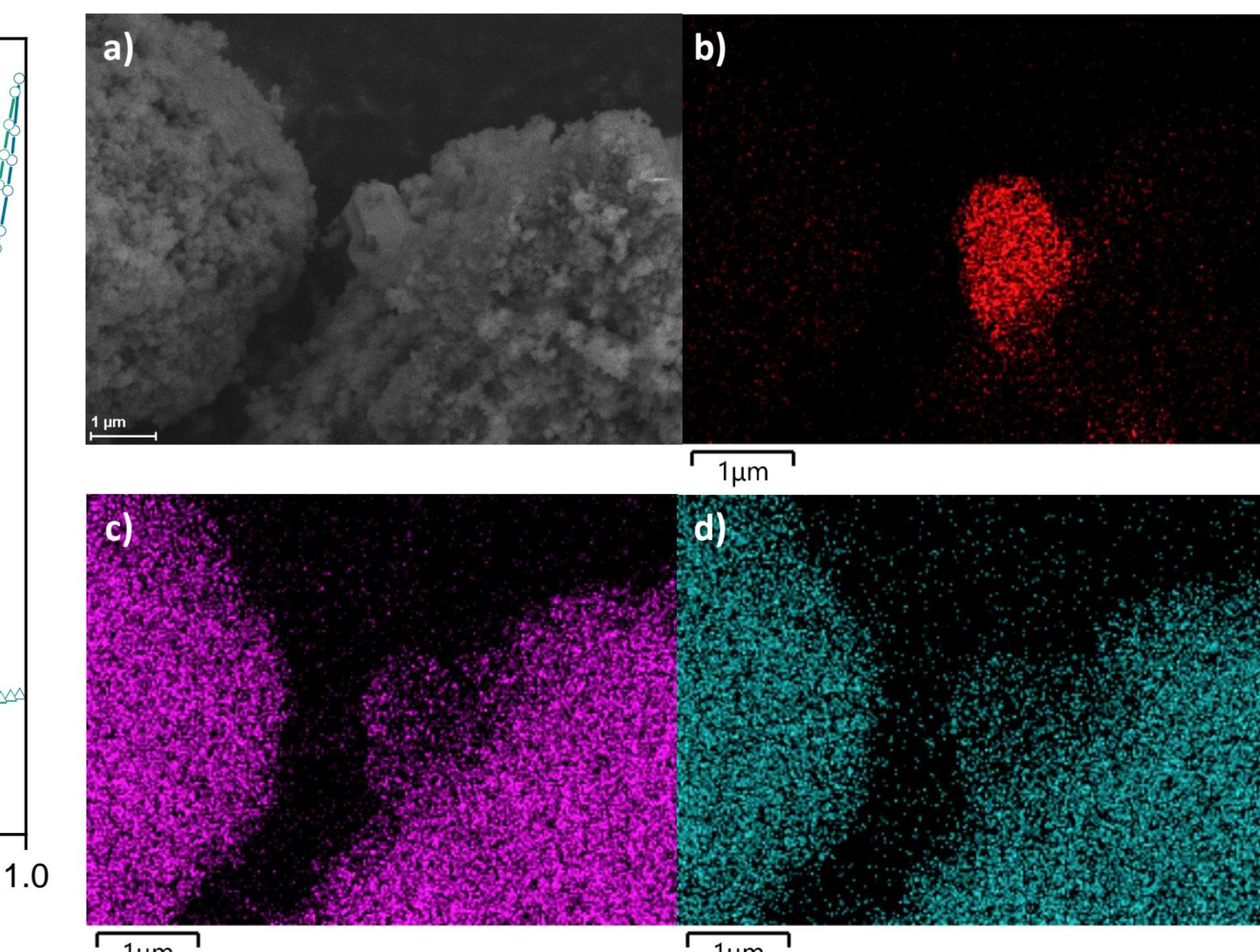
Figure 8: a) SEM image, b) Cu-, c) Si-, and d) Mg-energy dispersive X-ray (EDX) mapping of Mg-Saponite impregnated with Cu; EHT = 5–20 kV, WD = 10.0 mm, magnification 20,000.
