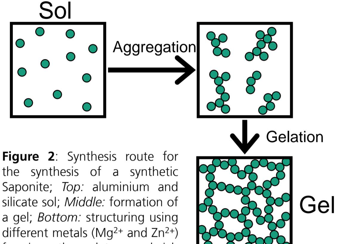
Figure 2: Synthesis route for the synthesis of a synthetic Saponite; Top: aluminum and silicate sol; Middle: formation of a gel; structuring using different metals ( $Mg^{2+}$  and  $Zn^{2+}$ ) forming the platy sandwich structure of saponites.<sup>[5-7]</sup>
