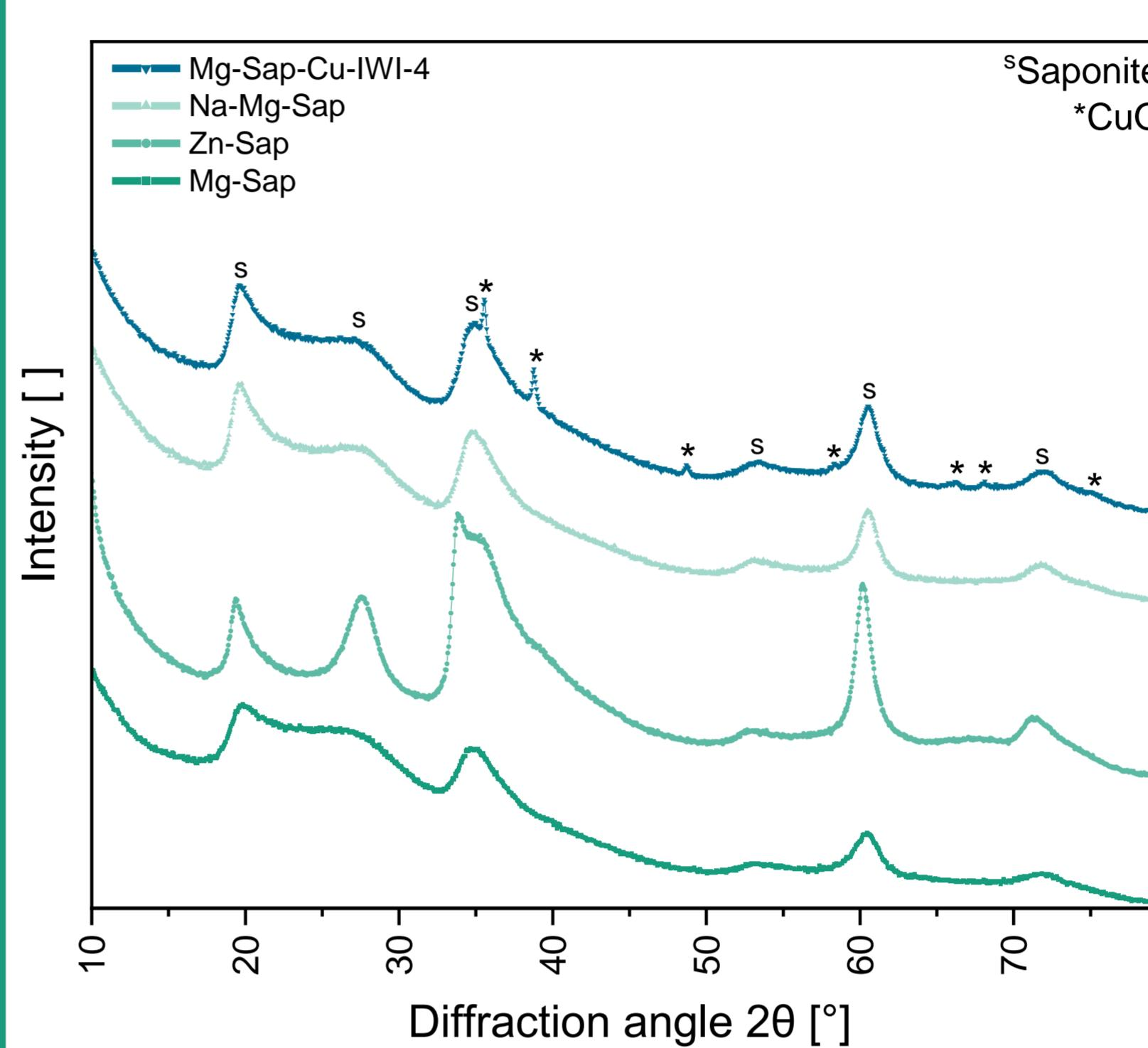
Figure 4: X-ray diffraction (XRD) pattern of the different synthesized catalysts. Reflexes marked with 's' corresponds to the saponite structure<sup>[5]</sup>; '\*' marked reflexes to  $CuO$ <sup>[8]</sup>.
