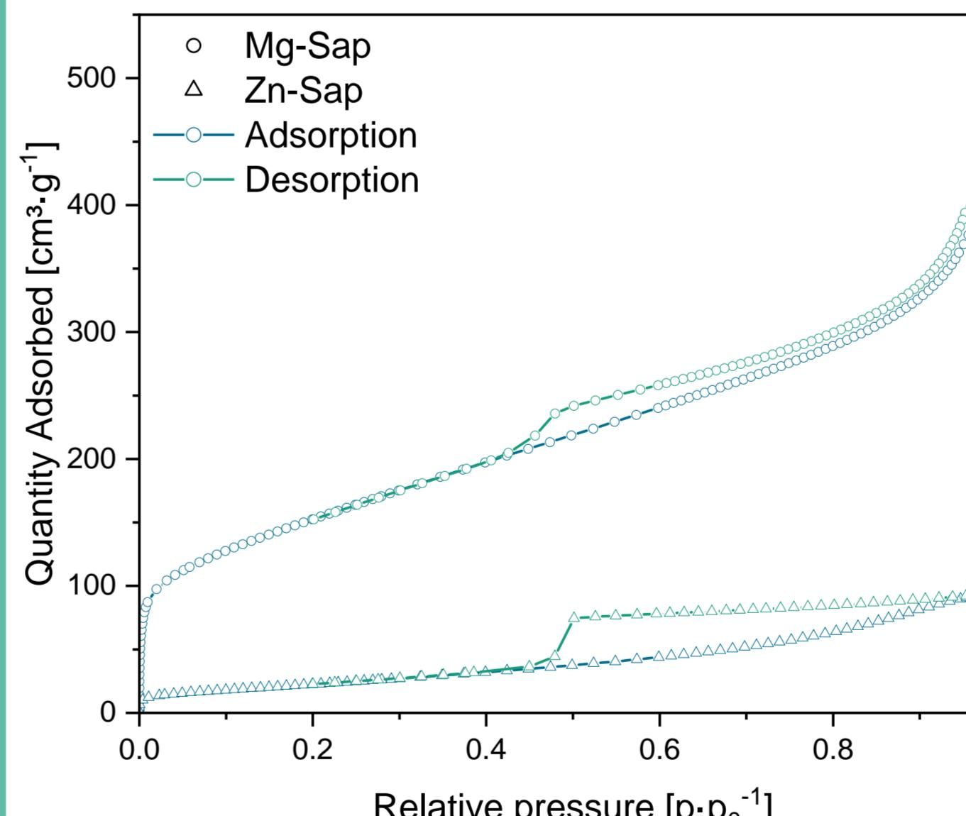
Figure 6: Top: Table with BET-surface areas of the catalysts; Bottom:  $N_2$  adsorption-desorption curves of Mg- and Zn-Saponite.
