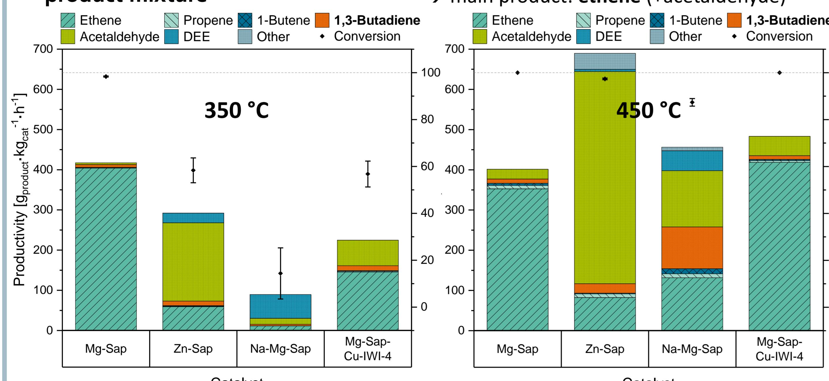
Figure 9: Product productivities in the ETB reaction using different catalysts;  $\dot{V}_{(total)} = 100 \text{ mL} \cdot \text{min}^{-1}$ ,  $c(\text{Ethanol}) = 4.6 \text{ mol\%}$ ,  $p_{\text{absolute}} = 1 \text{ bar}$ , WHSV = 1  $\text{h}^{-1}$ .
