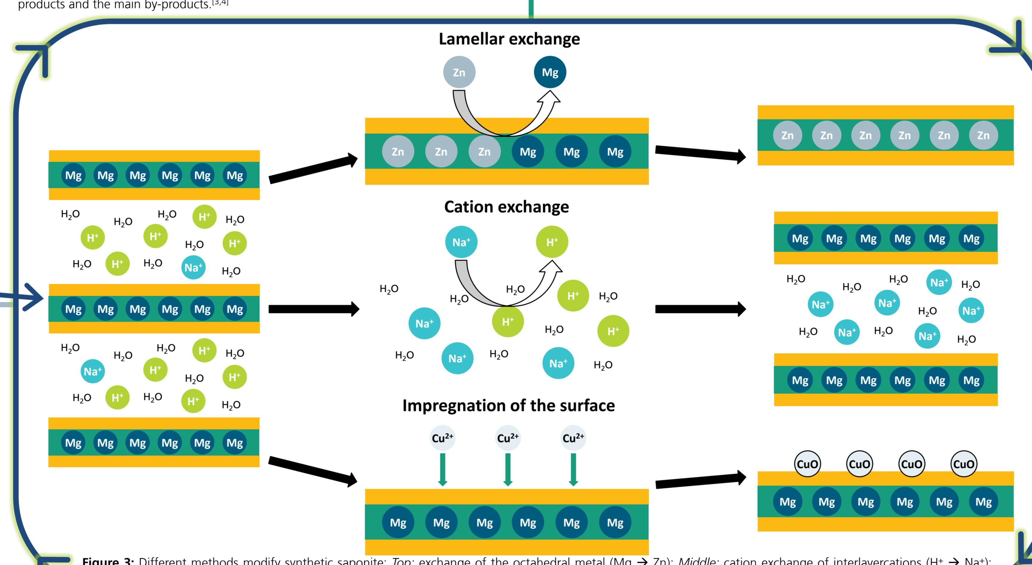
Figure 3: Different methods modify synthetic saponite; Top: exchange of the octahedral metal ( $Mg \rightarrow Zn$ ); Middle: cation exchange of interlayer cations ( $H^+ \rightarrow Na^+$ ); Bottom: loading of a synthetic Mg-Saponite surface with  $CuO$  (Surface— $CuO$ ).
