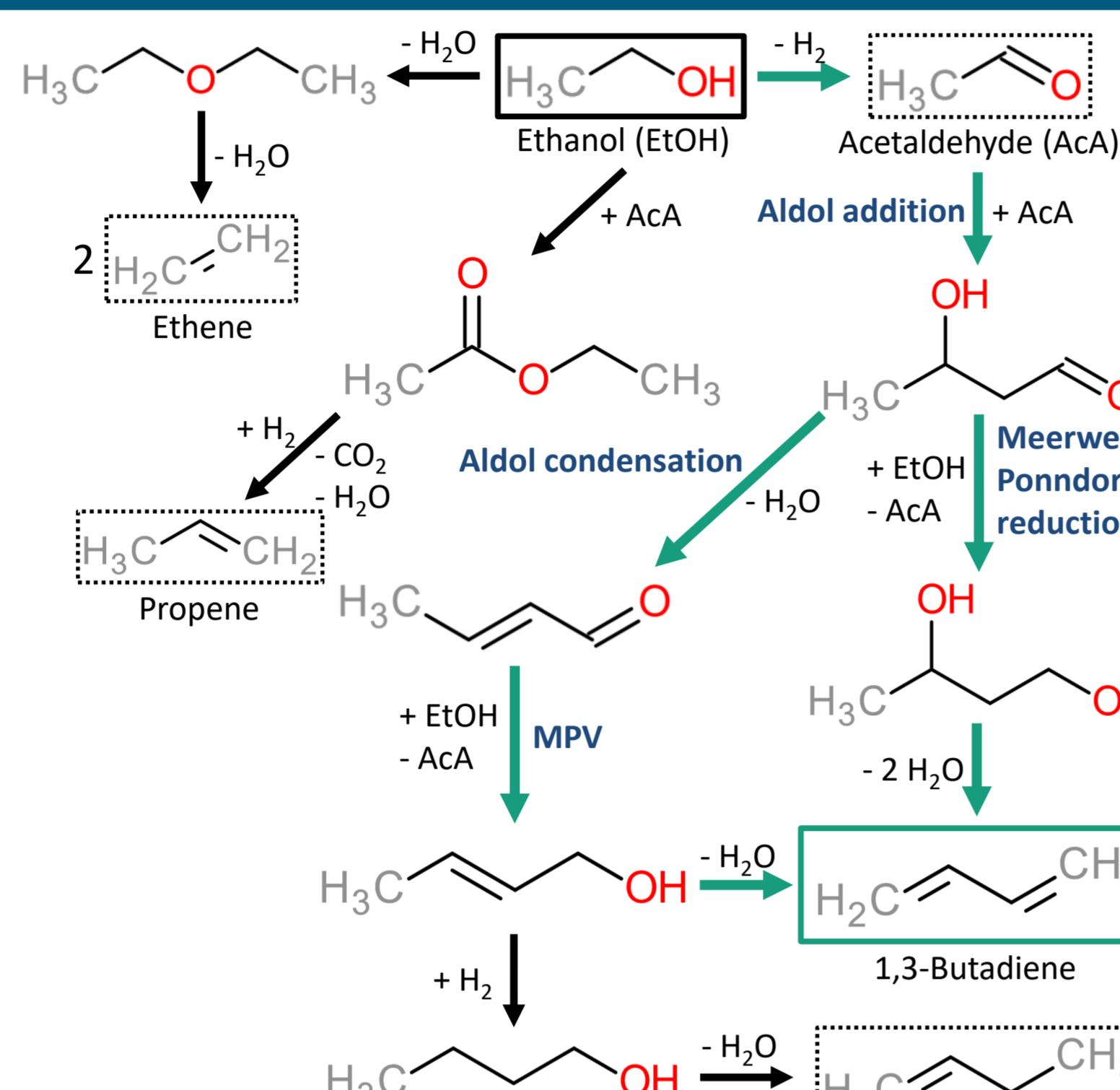
Figure 1: Reaction scheme for the reaction of ethanol to 1,3-butadiene with intermediate products and the main by-products.<sup>[3,4]</sup>
