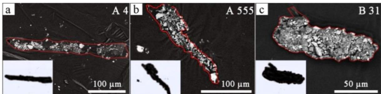
Fig. 1 Scanning Electron Microscopy pictures of typical super-coarse TRWP particles from motorways [10]
