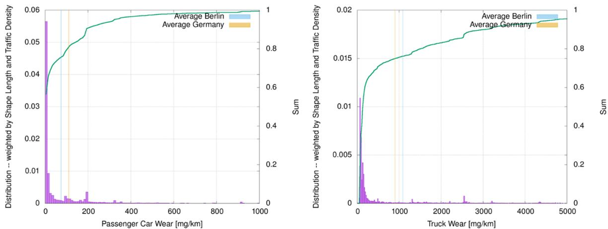
Fig. 3 Distribution of the TWP per vehicle kilometer. The distribution is weighted by shape length and traffic intensity
