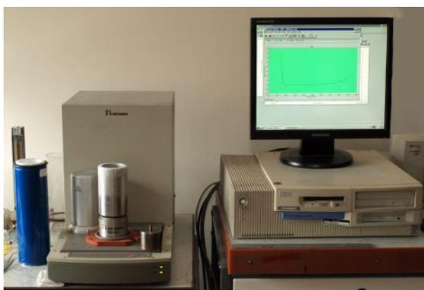
The DSC analysis is used to study phase transitions or chemical reactions.
