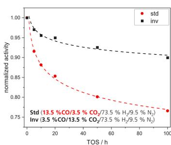
Figure 1: Induction of the commercial methanol synthesis catalyst in clean synthesis gas of different compositions.
