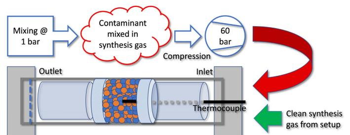
Figure 2: Conceptual design of the long term dosing experiment – Catalytic test setup with two separate and switchable synthesis gas mixing sections.
