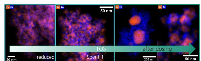
Figure 4: EDX maps of different catalyst lifetime stages – a) reduced catalyst, b) catalyst induced for 24 h TOS and c) spent catalyst after oxygen dosing and recovery in clean synthesis gas.
