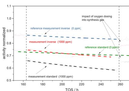
Figure 3: Oxygen poisoning during methanol synthesis – 1,000 ppm O<sub>2</sub> dosed into syngas after induction for 100h.
