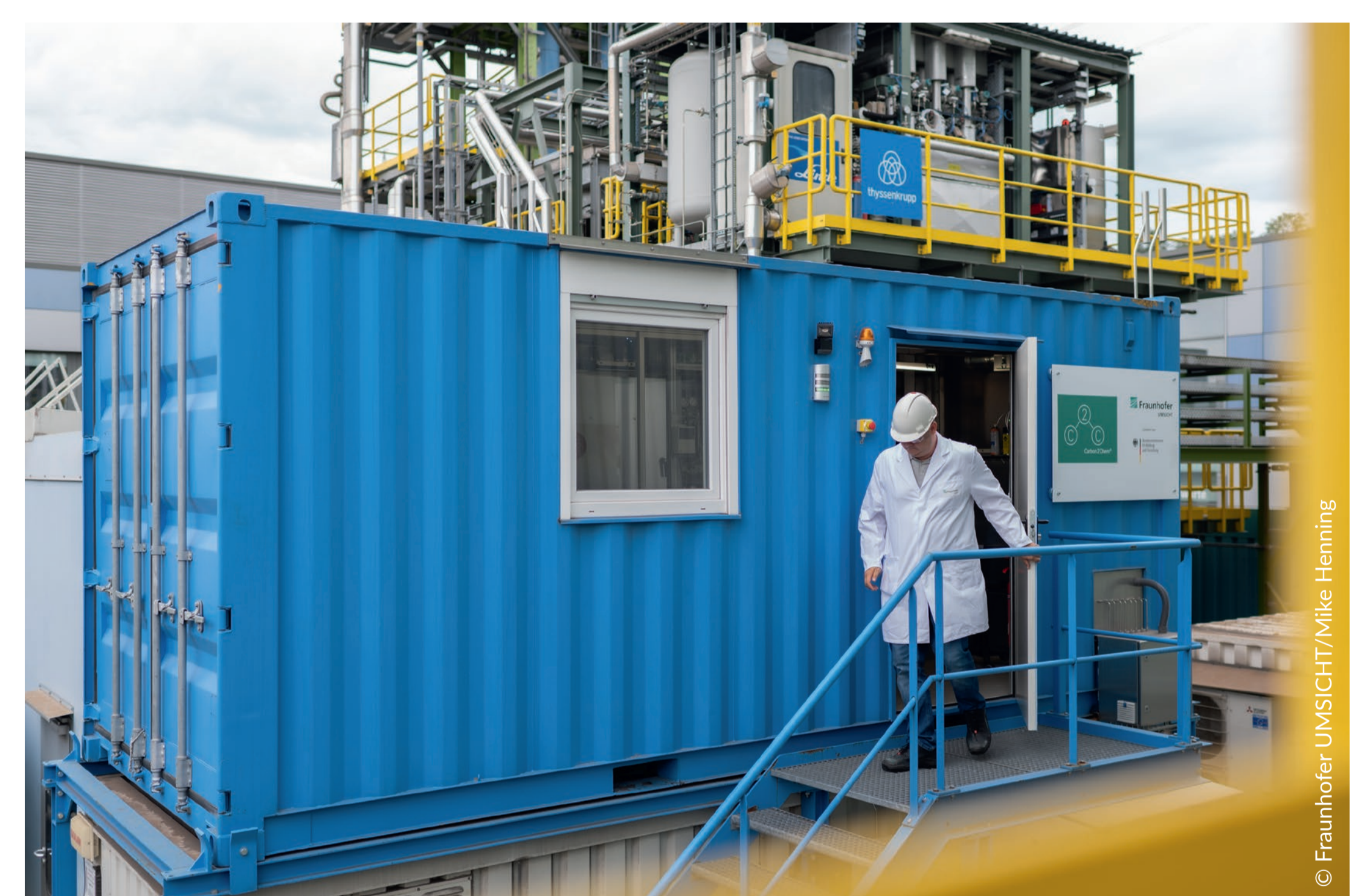
Test system is transportable by using a container set up
