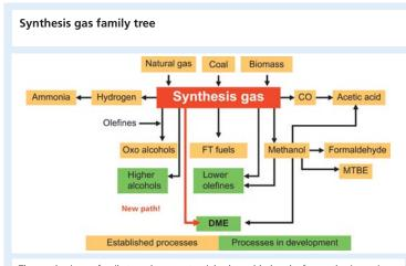
The synthesis gas family tree shows potential value added paths for synthesis gas in accordance with the roadmap of the German Catalysis Society (Deutsche Katalyseforschung), GECATS, March 2010
