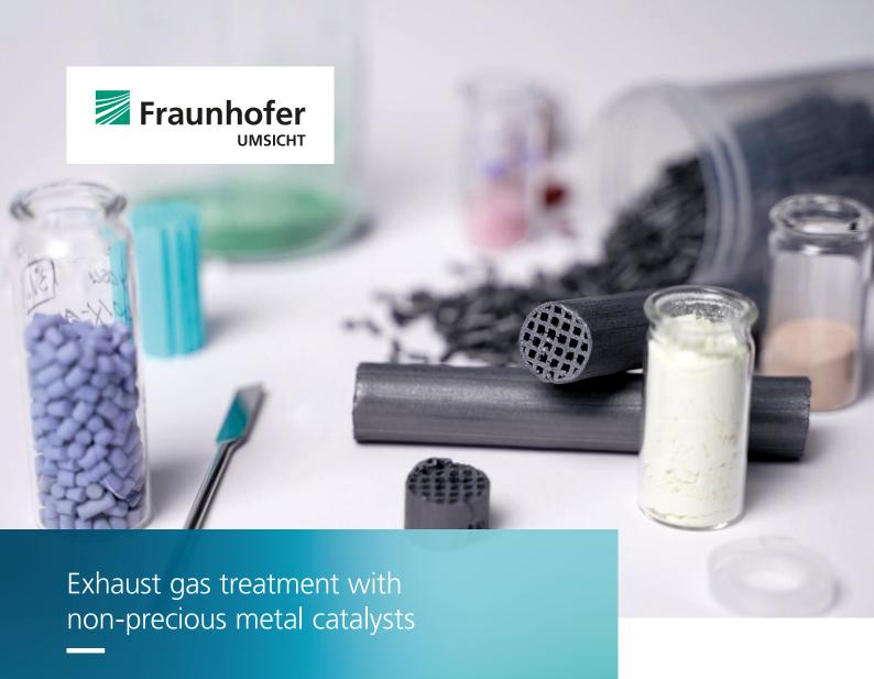
Methane oxidation catalysts for gas engines
