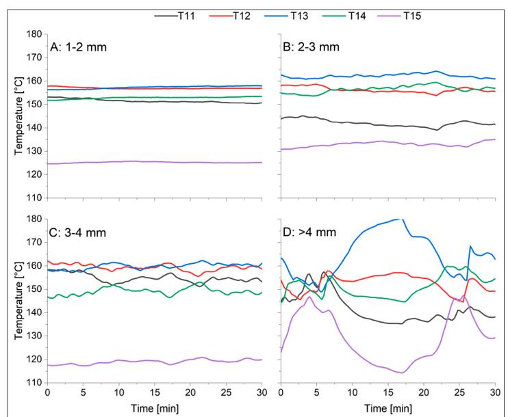
**Fig. 2:** Temperature distribution of the four particle sizes (A-D) during heating experiments (T11: top; T15 bottom).
