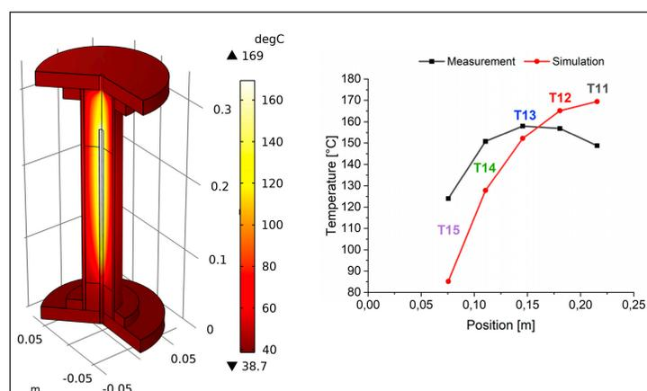
**Fig. 1:** a) Simulated temperature distribution of the whole setup considering e.g. natural convection, electrical heating, gas flow and material properties.
