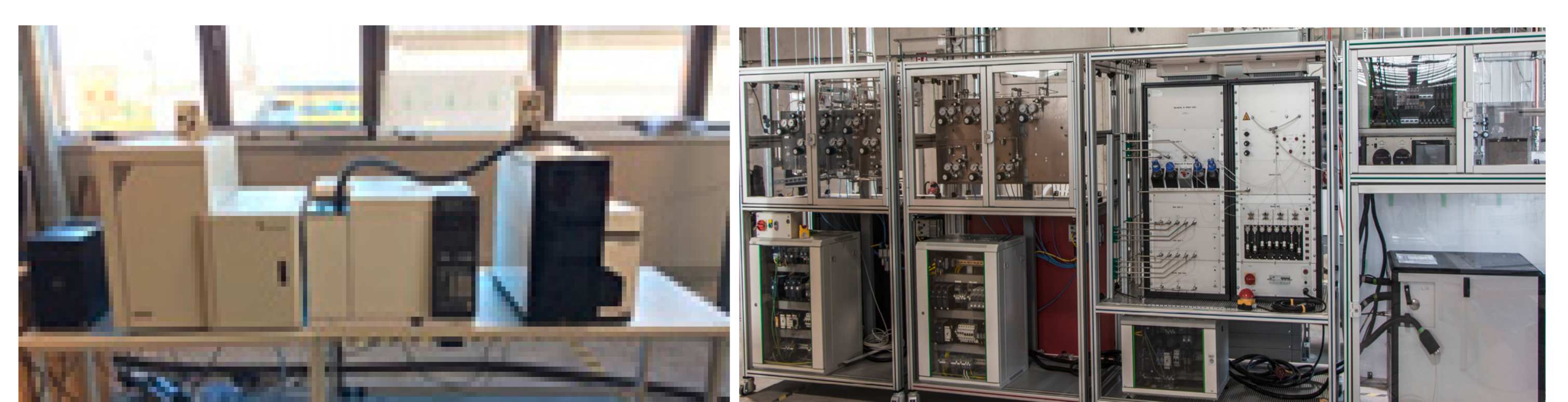
Figure 5 TD-GCMS (left) and calibration gas generator (right) used for method validation in Carbon2Chem®-Laboratory (Oberhausen).
