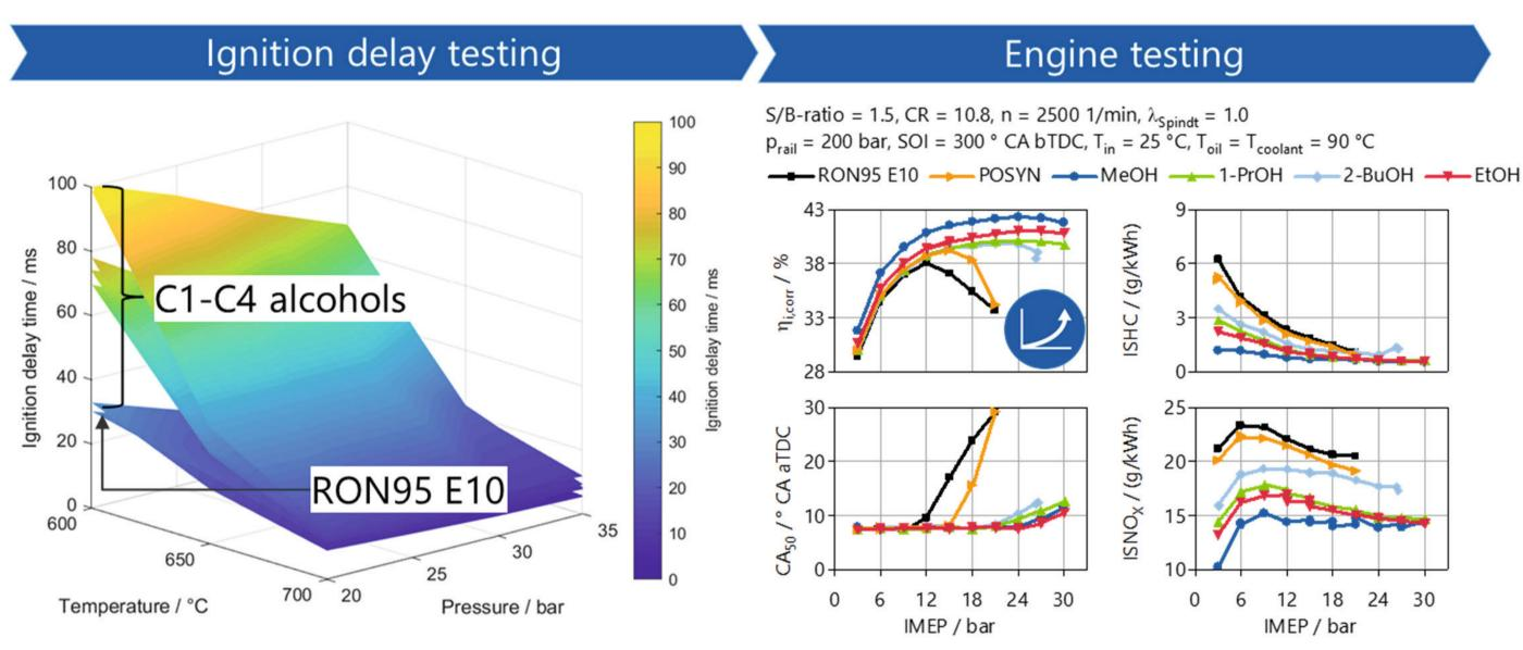
Ignition delay and engine testing of  $C_1$ - $C_4$  alcohols vs. gasoline.
