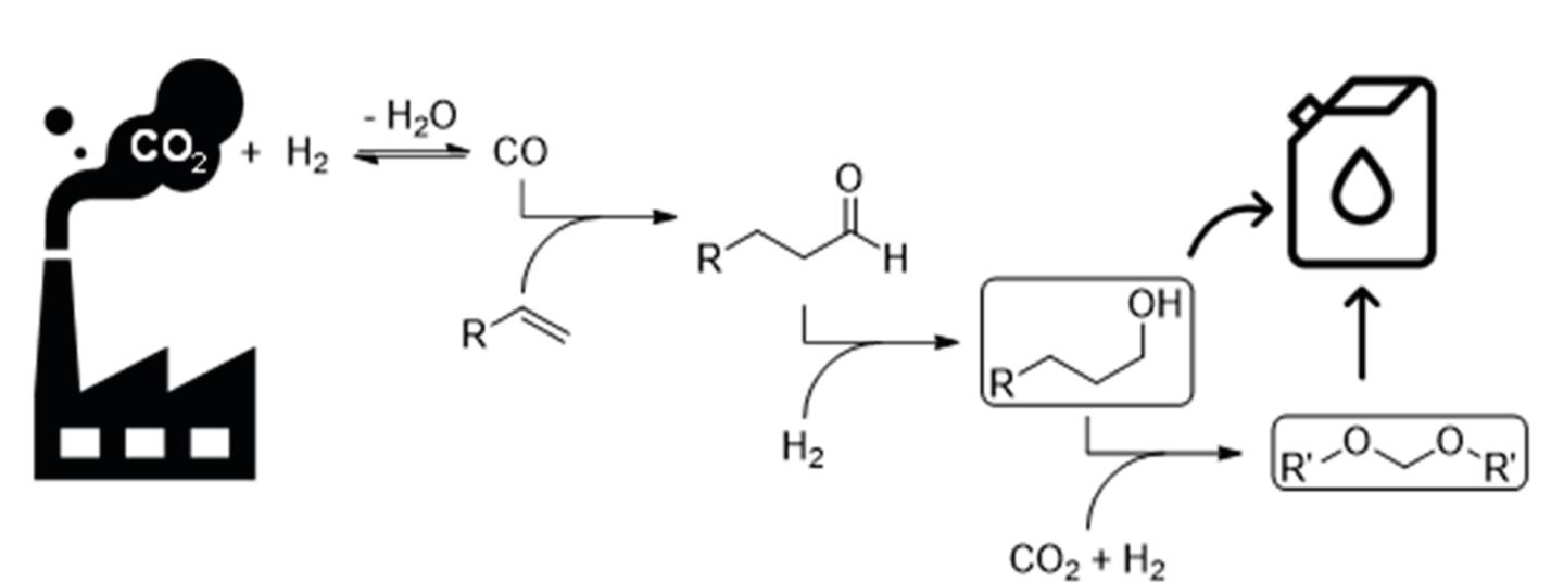
Reverse water-gas shift based access to alcohols and acetals.
