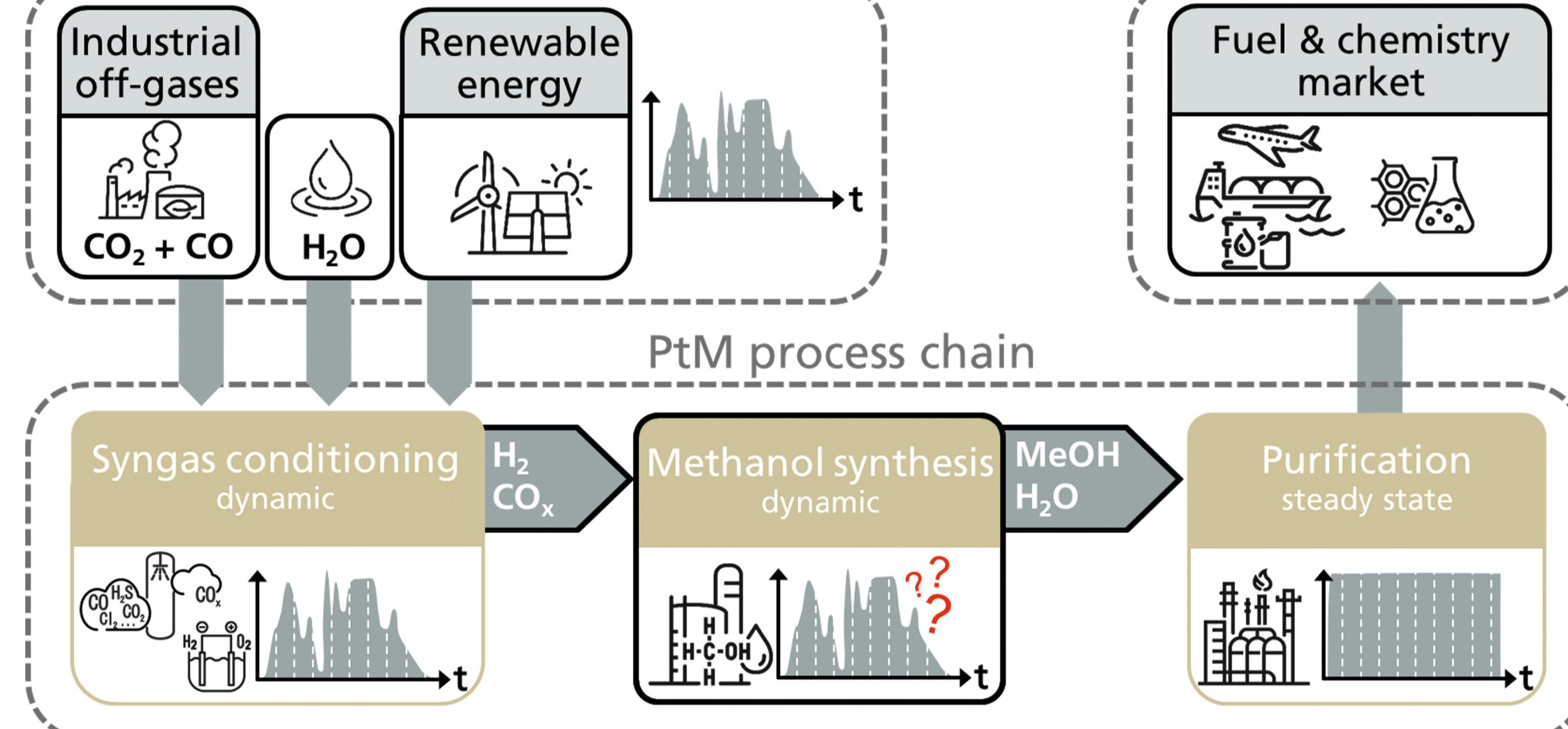
Fig. 1: Schematic illustration of PtX process chain via the dynamically operated methanol synthesis
