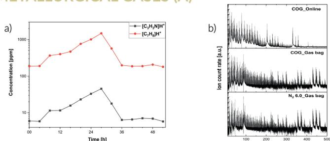
Figure 2: a) Time series of toluene and acrylonitrile in raw coke oven gas using  $H_3O^+$  as primary ion. b) Full mass spectra of coke oven gas and nitrogen 6.0 measured online with PTR-QiTOF. [1]
