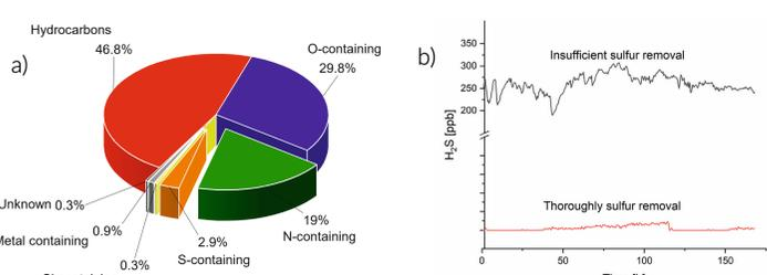
Figure 3: a) Gas composition of the treated BFG measured via Proton Transfer Mass Spectrometry (PTR-MS). b) Comparison of an insufficient and a thoroughly sulfur removal via the gas treatment in Carbon2Chem®. [2]
