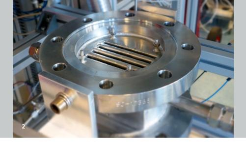
**2** Reactor for producing long-chain alcohols using the Fischer-Tropsch process.
